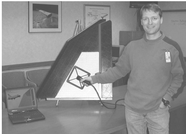
Figure 4. Demonstration of rapid communication with many RFID tags at 125 kHz using anti-collision technology.
