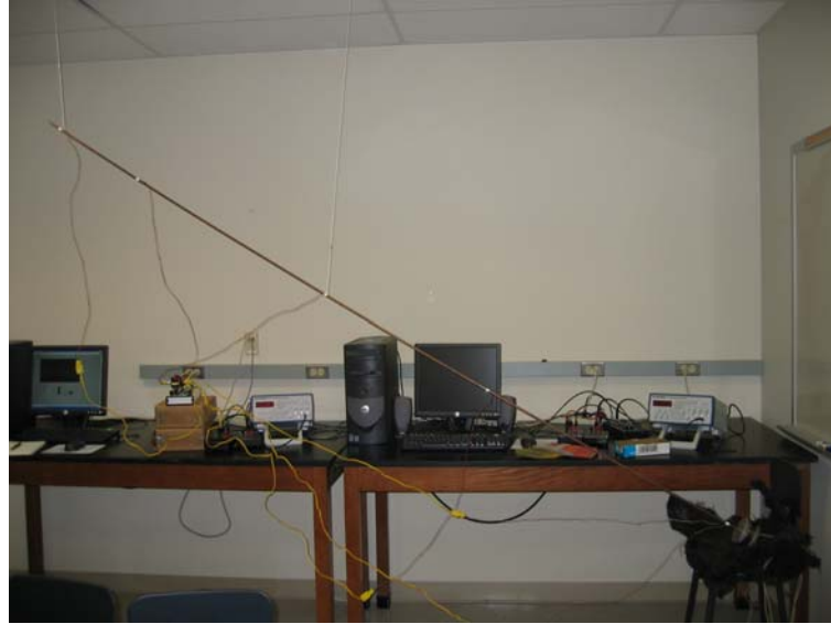
Figure 5: 10' Supertubes Figure 6: Setup for band heater testing of 10' Supertubes
