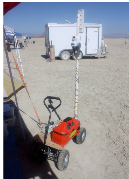
Figure 7. Mobile Cart with Radio, PTZ Video Camera and Power.
