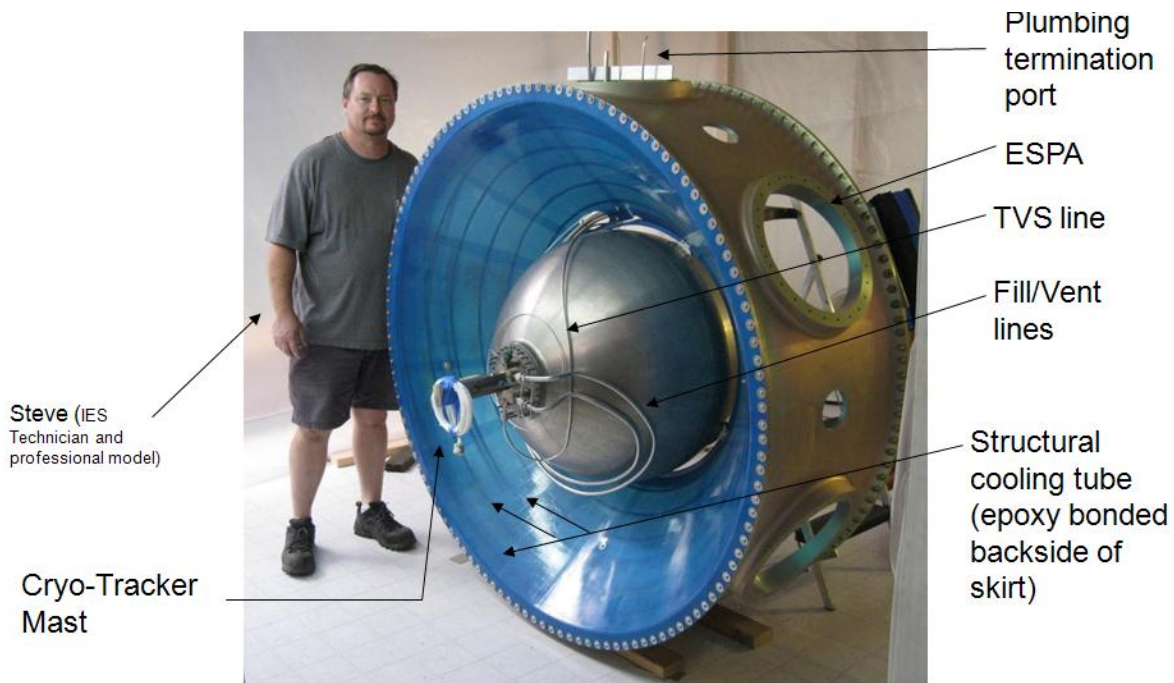
Figure 2: CRYOTE Ground Test Article and Instrumentation (excluding MLI)
