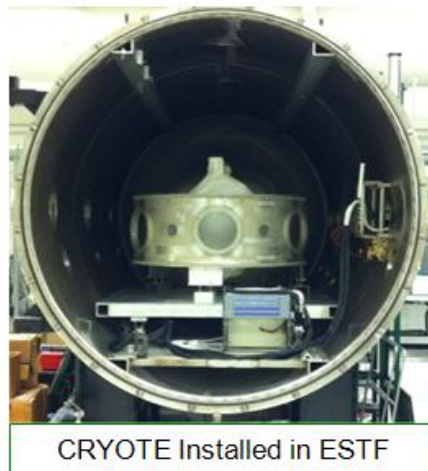
Figure 4: CRYOTE GTA Installed in ESTF Vacuum Chamber
