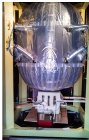
Figure 8: EDU tank as installed in TS 300.
