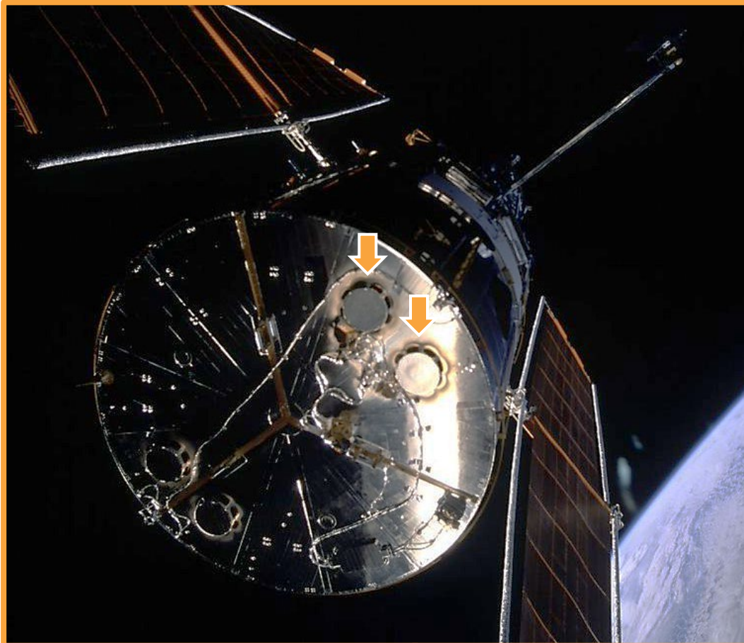
Silver Teflon tape near aft vents on the Hubble Space Telescope (HST)
