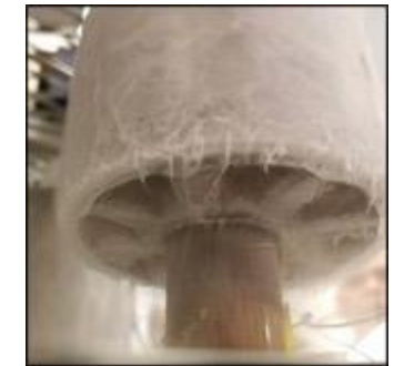
Cryofreezer cold-head concepts and modeling (top); cold-head installed on test stand (bottom left); CO 2 ice accretion
