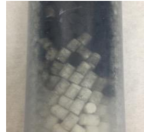
Post-vibration testing showing catalyst dust migration
