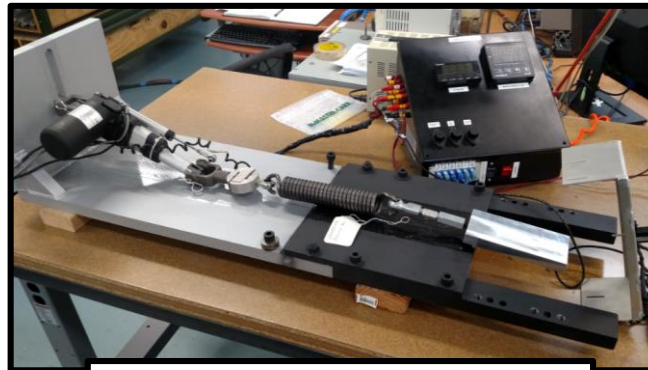
Retention testing apparatus with linear actuation and control box for clamp testing
