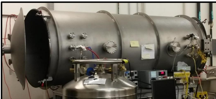
ACT thermal vacuum chamber for testing at lower than atmospheric pressure and for simulation of spacecraft conditions.
