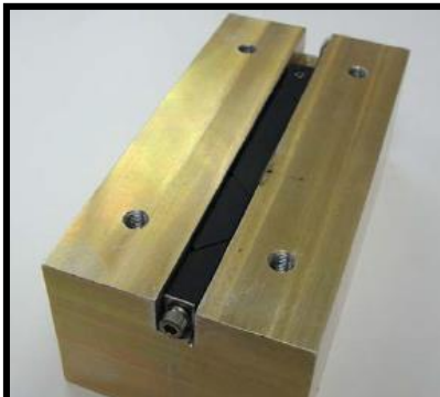
Lockheed Martin test setup for mechanical cycling of a card lock device.
