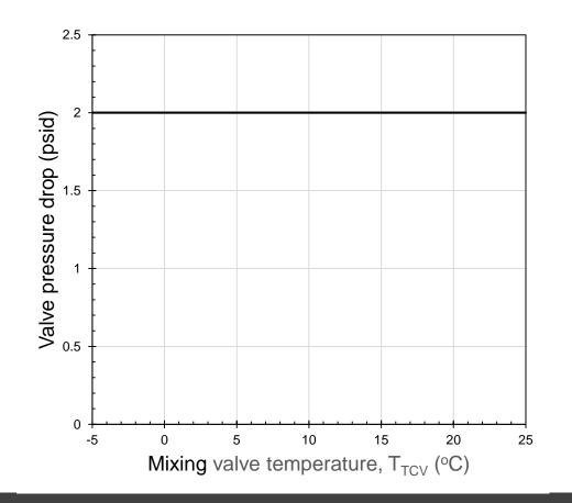
Resulting impedance curve based on spec. of minimum 4% flow increasing linearly to 96% between 0 °C and 20 °C
