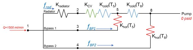
Thermal model uses flow fractions from fluid model to determine fluid temperatures
