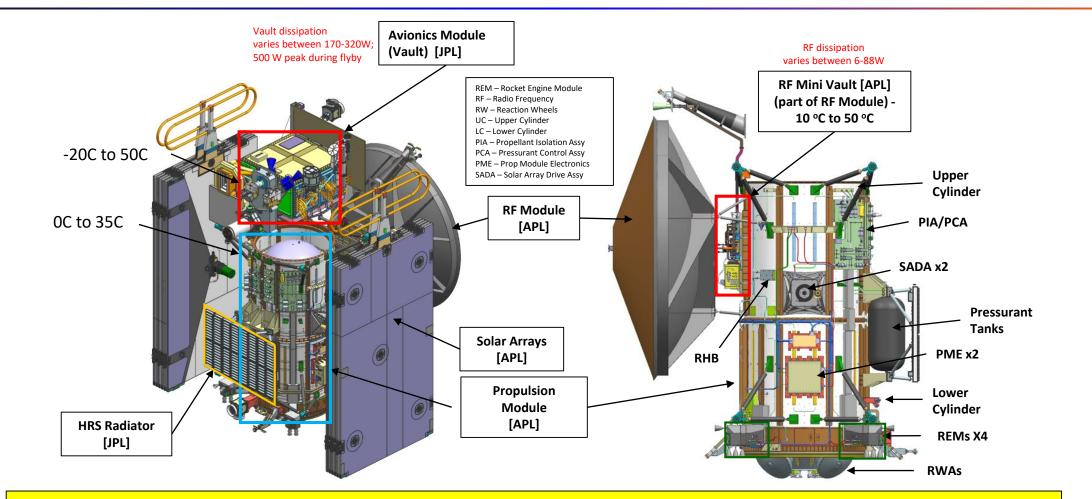
Europa Clipper has a mechanically pumped fluid loop (MPFL) that harvests heat from the e-boxes in the Vault and dissipates the heat to the propulsion components or out the radiator when vault dissipation is too large
