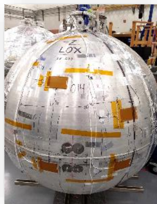
PZT patches bonded To LOX tank
