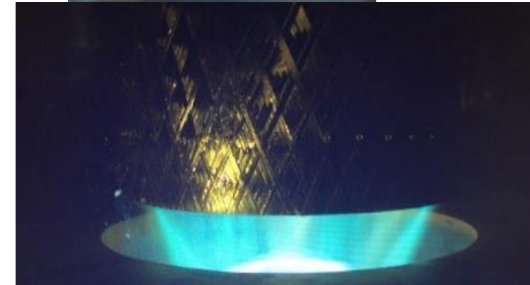
7000 gal water tank, feeds diffuser cooling spray bars. Enters chamber through upper personnel door.
