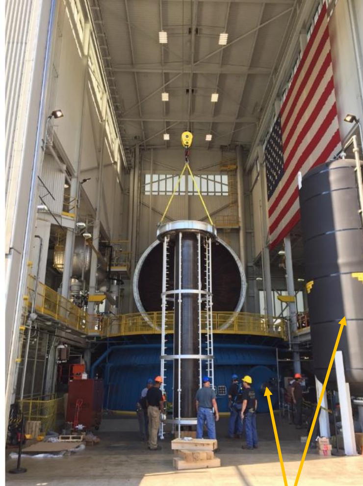
7000 gal water tank, feeds diffuser cooling spray bars. Enters chamber through upper personnel door.
