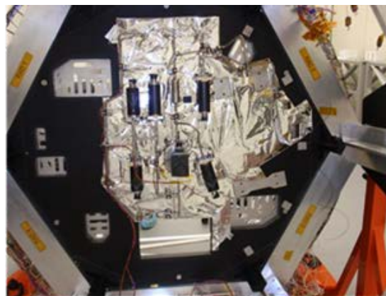
Underside of Top Deck with partial MLI installed (Faces toward inside of spacecraft)
