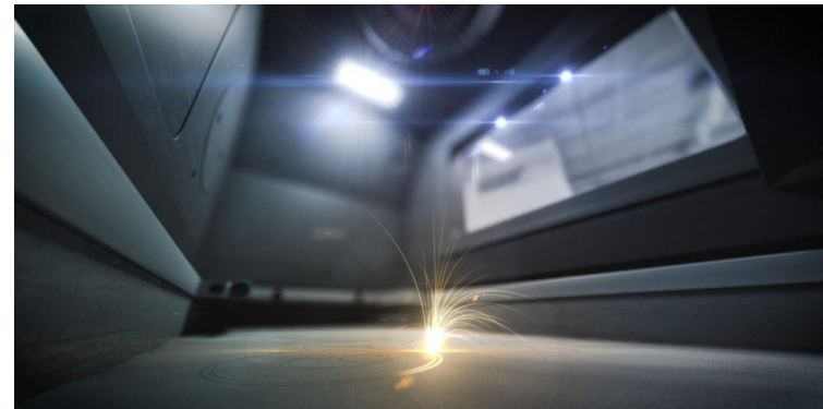
[2] Selective Laser Melting process on metal powder bed
