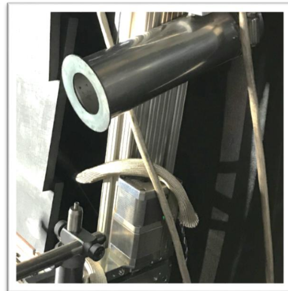
Collimator mounted in vacuum chamber
