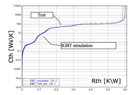
• From here the package thermal metrics can be identified accurately using simulation
