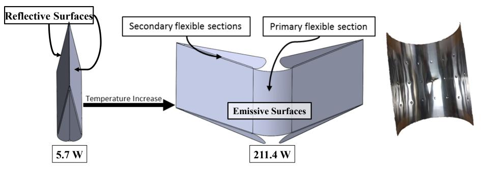
NASA Roadmap: Looking for Variable Geometry Radiators with a 6:1 turndown capability, with 12:1 as a stretch goal
