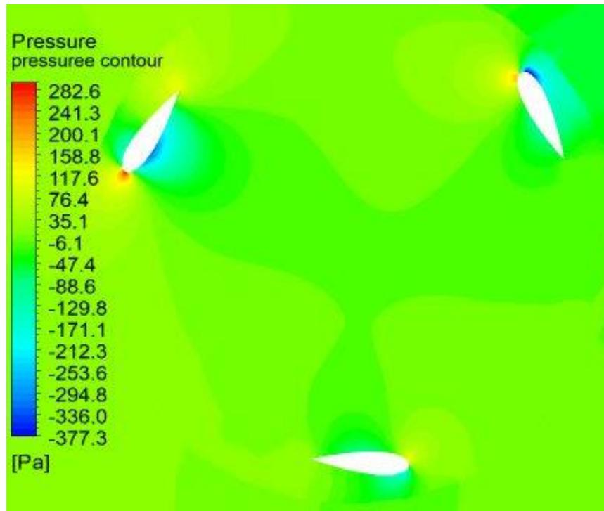
Figure 12 Darrieus pressure contour at TSR Of 1.8
