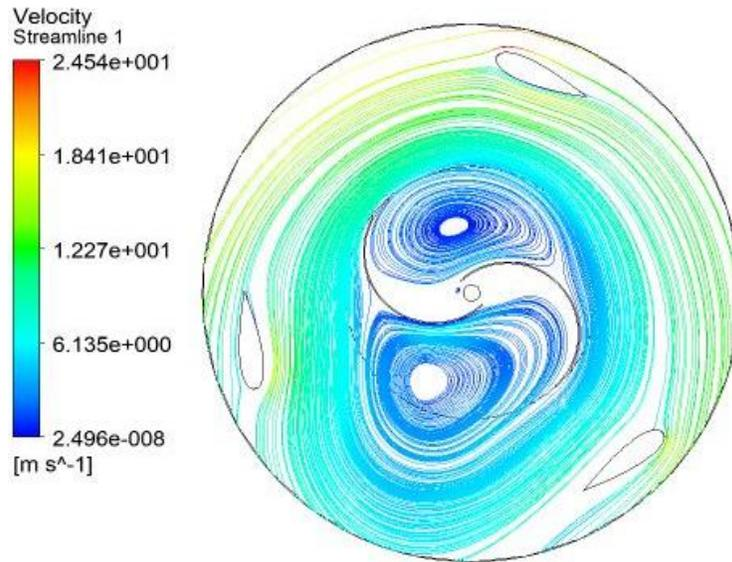
Figure 15 Hybrid particle tracking at TSR Of 1.8
