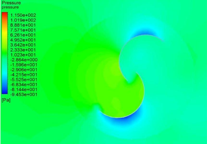
Figure 8 Savonius pressure contour at TSR Of 0.2
