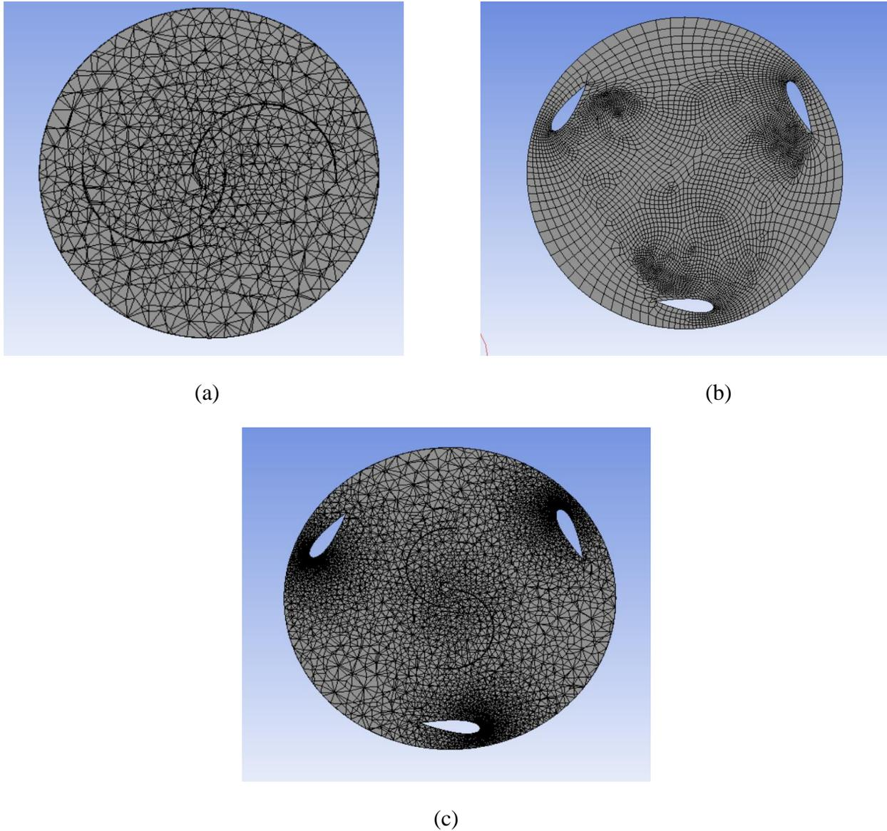
Figure 3 Meshing of different configurations (a) Darrieus, (b) Savonius and © Hybrid mesh.
