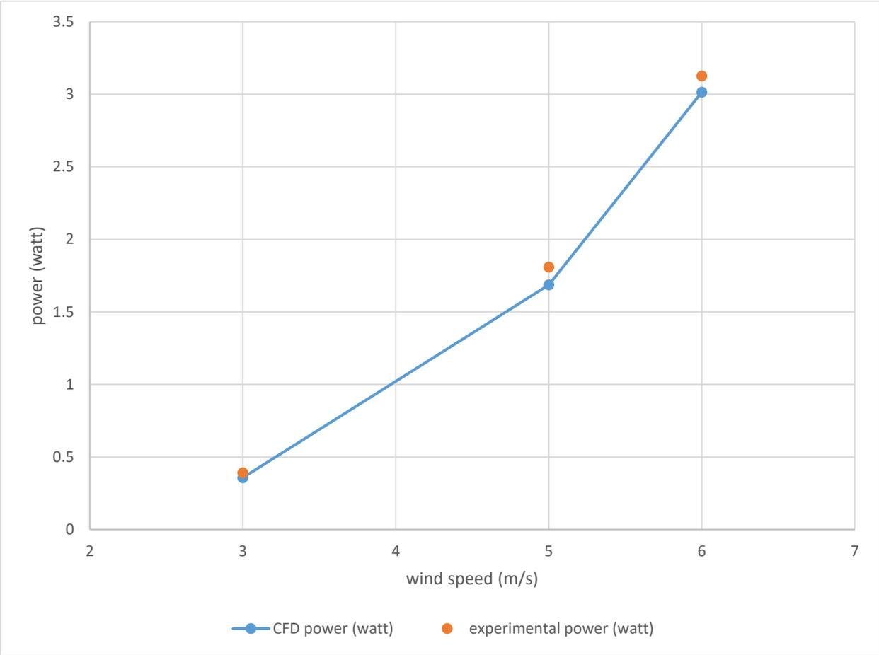
Figure 5 Comparison between the present numerical and experimental results of Siddiqui et al. [30, 31] for Savonius turbine
