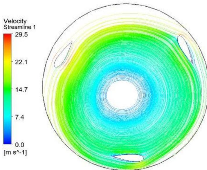
Figure 14 Darrieus particle tracking at TSR Of 1.8
