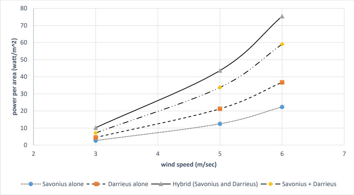
Figure 6 Comparison between variations of turbine output power per turbine frontal area at different wind speed.
