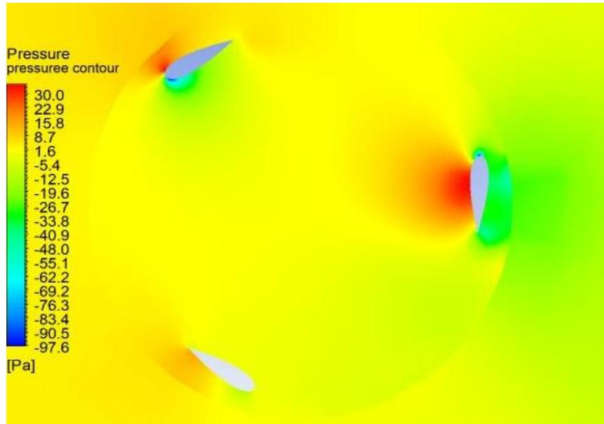
Figure 9 Darrieus pressure contour at TSR of 0.2
