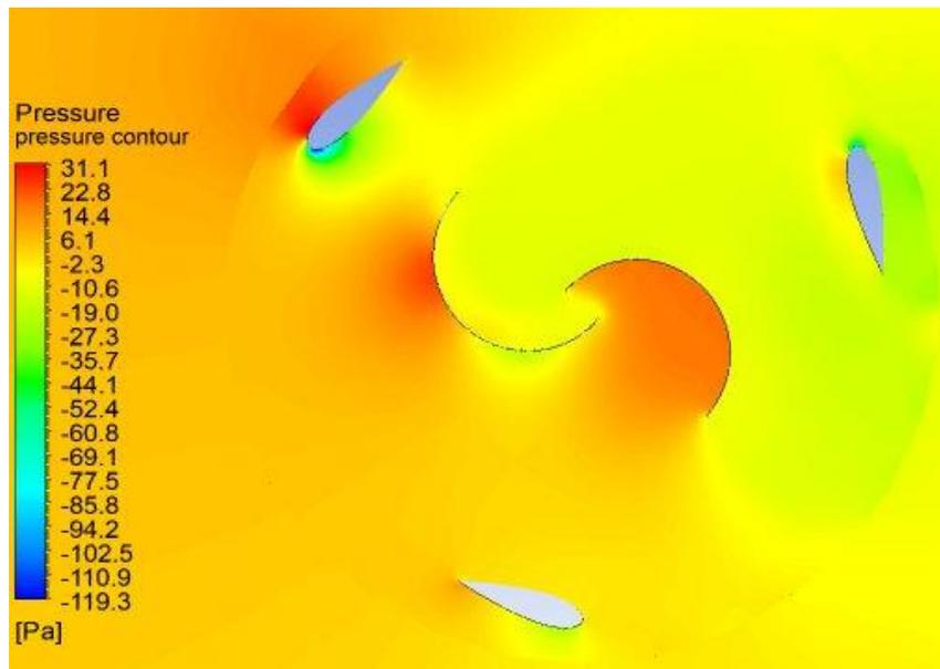
Figure 10 Hybrid pressure contour at TSR of 0.2
