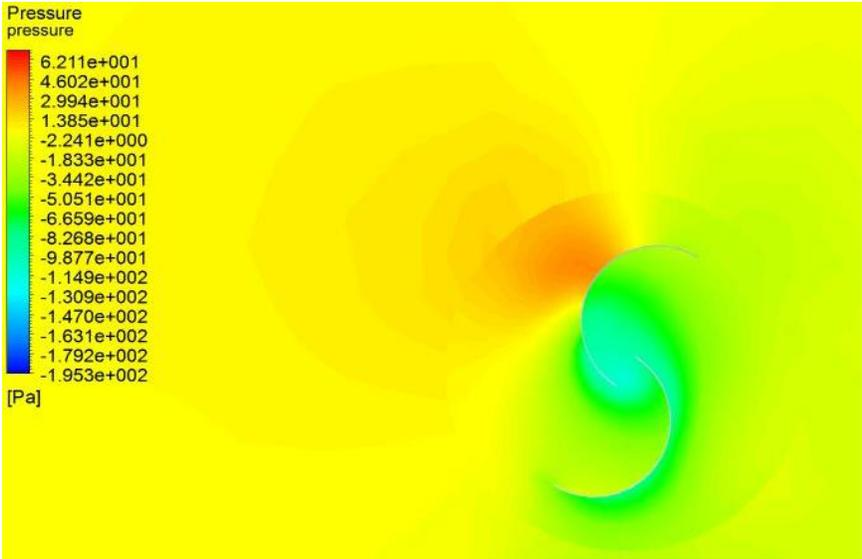
Figure 11 Savonius pressure contour at TSR Of 1.8
