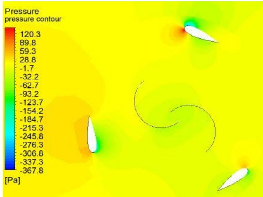
Figure 13 Hybrid pressure contour at TSR Of 1.8
