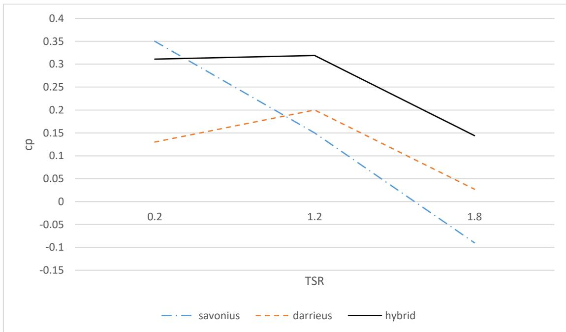
Figure 7  $C_p$  variation with the tip speed ratio
