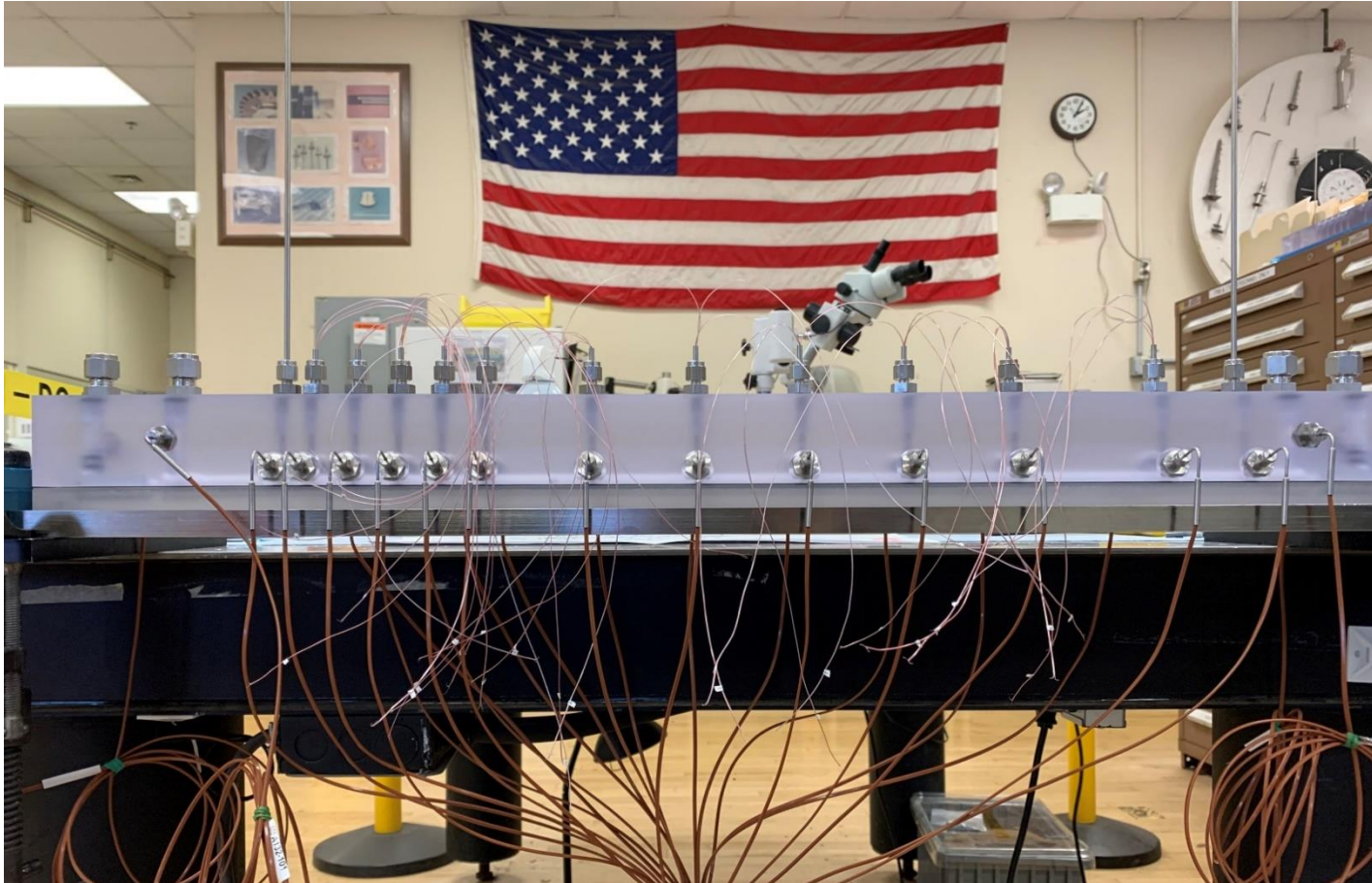
Condensation Test Module assembled polycarbonate Test Section
