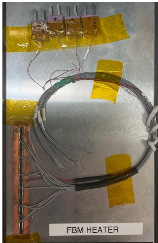
Mock-up of the Flow Boiling Test Module copper strip heaters
