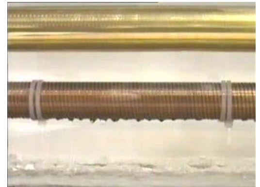
induction pumping of external condensation
