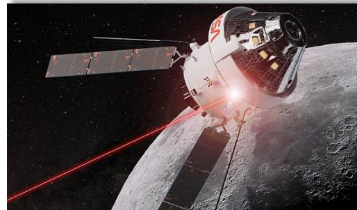
Laser Communications Terminal for Artemis II NASA GSFC, MIT Lincoln Lab, Lockheed Martin https://www.nasa.gov/feature/goddard/2022/the-future-of-laser-communications
