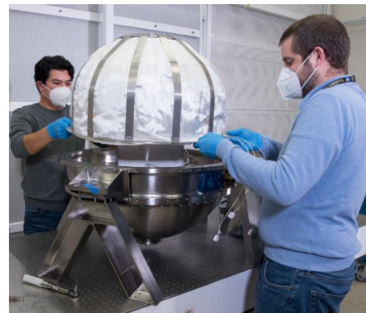
Aft Insulation and Retainer
