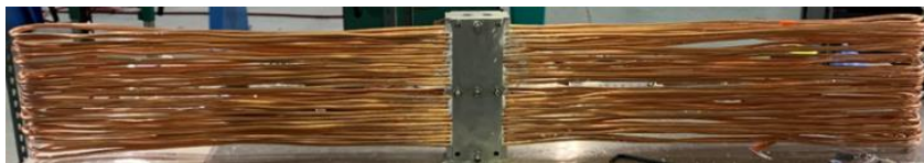
44" long copper bent tube OHP Photograph taken prior to silicone-ceramic black coating
