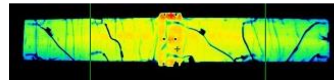
IR image of flat plate OHP radiator operating at ~175-deg C at ThermAvant Technologies
