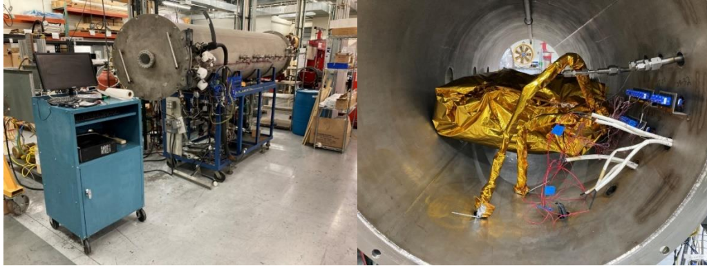
Figure 10. Thermal Vacuum Chamber, with Loop Heat Pipe Mounted Inside
