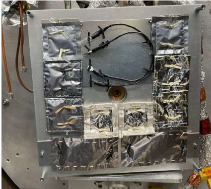
Figure 2. Radiation test setup with sample blankets and ground straps.
