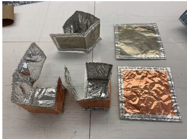
Figure 7. Small scale manufacturing samples with copper and stainless steel foil outer layers and PTFE coated fiberglass/Inconel sewing thread.
