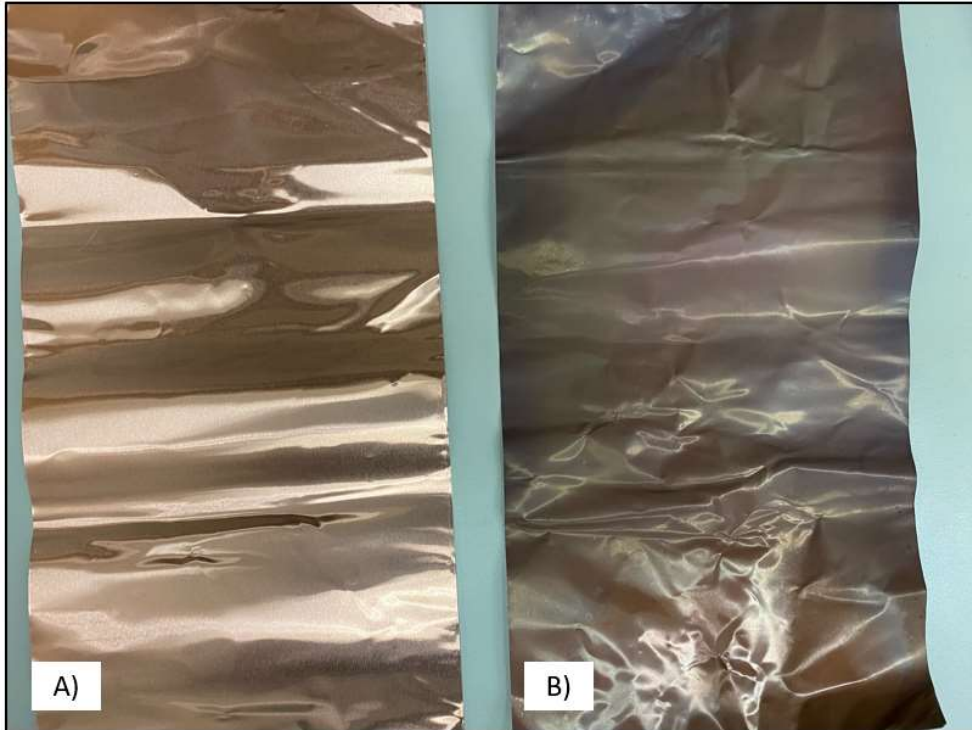
Figure A1. Copper foil A) pre test B) post test.
