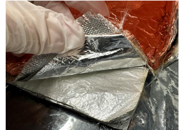
Aluminum, glass tissue separator layers
