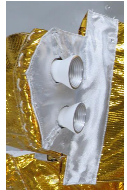
High temperature MLI patch with Nextel 312 flown on AMR-SWOT
