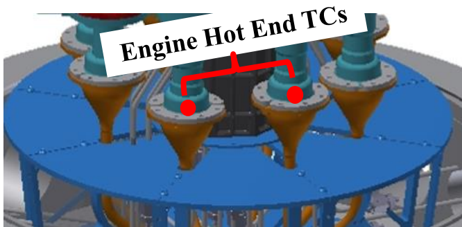
Delta T noted between Engine Hot End and adiabatic section of Heat Pipe
