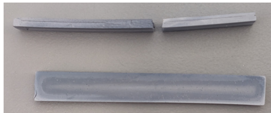
Figure 5: Sintered aluminum nitride beams, showing some oxidation and delamination.
