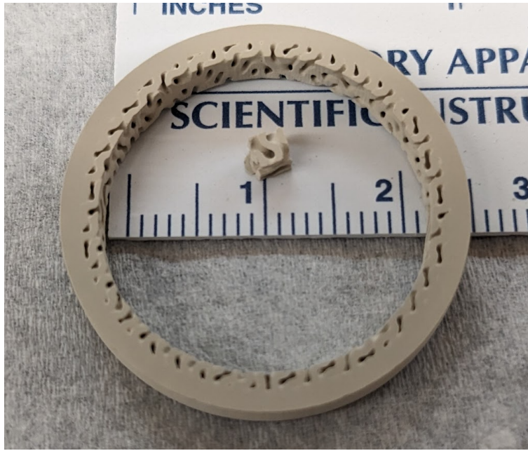
Figure 7: Optimized print settings, balancing print quality, interlayer adhesion, and print time produce high quality parts with fine feature definition.
