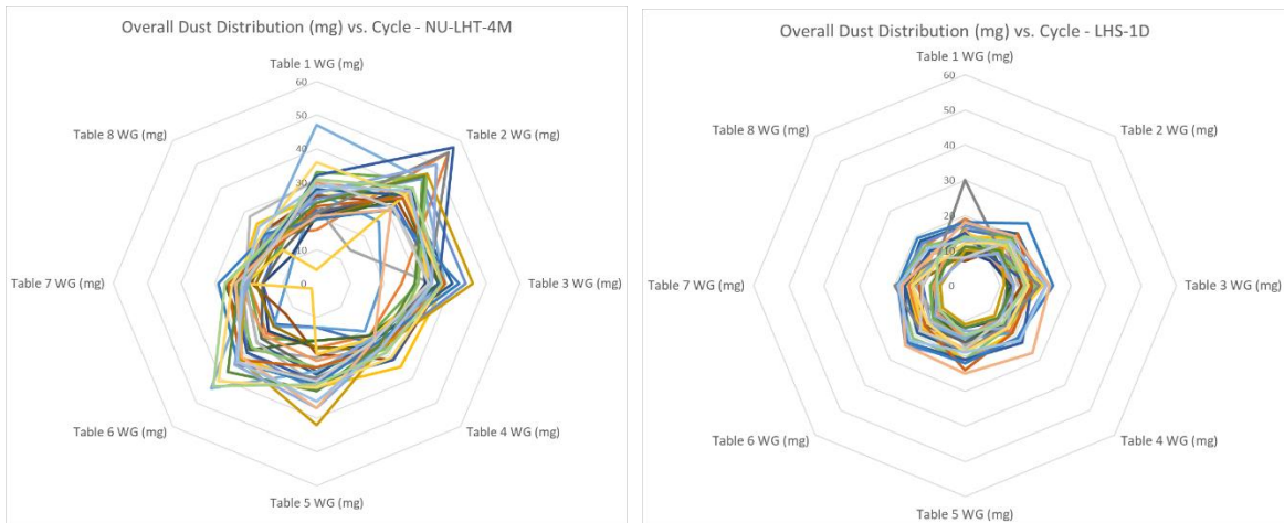
Figure 6. Radar graphs display the dust distribution across all 8 test tables for each cycle of dusting. Measurements are in mg and each graph contains 30 cycles worth of data.
