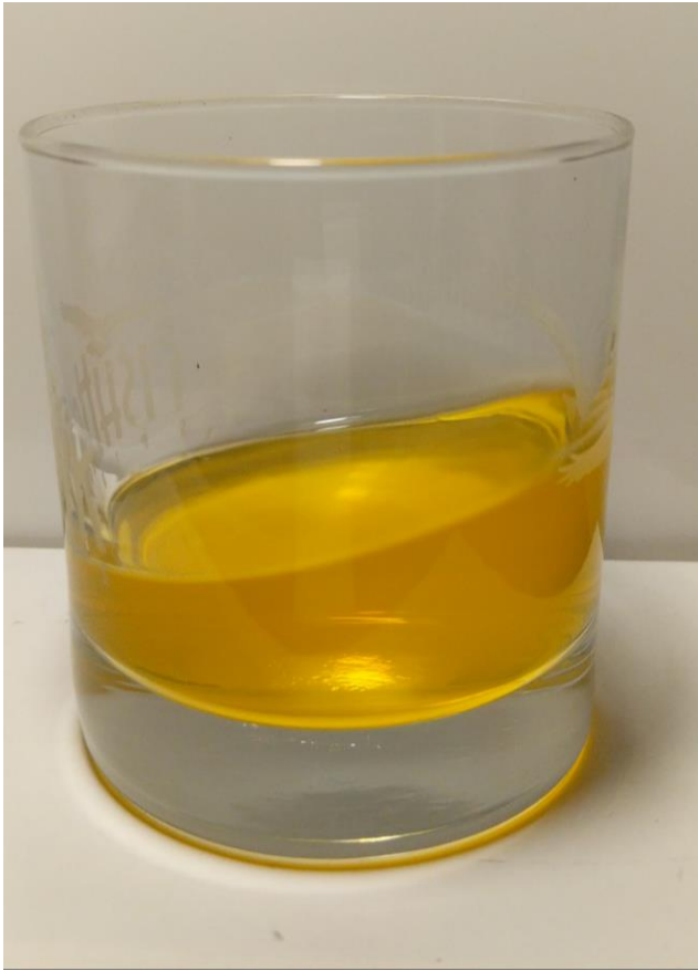
Natural frequency (the oscillating or sloshing yellow colored water in a glass) – Nevin Brosius
