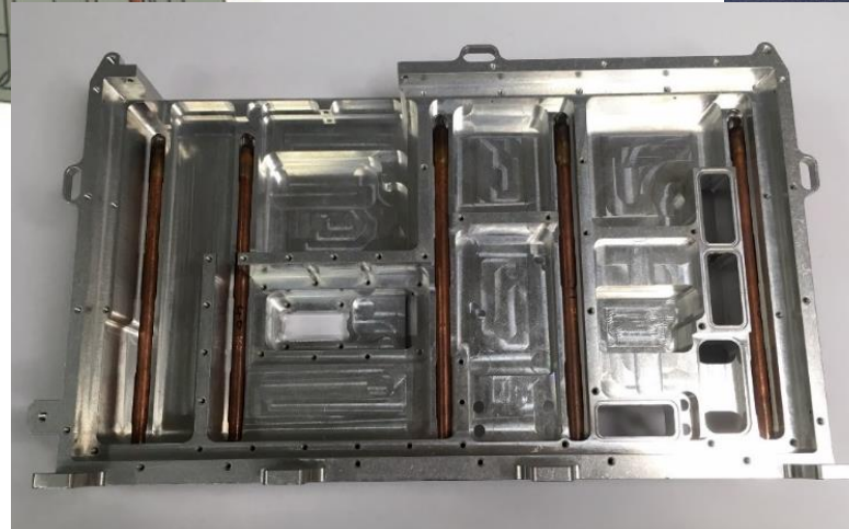
Cold Plate with Embedded Heat Pipes
