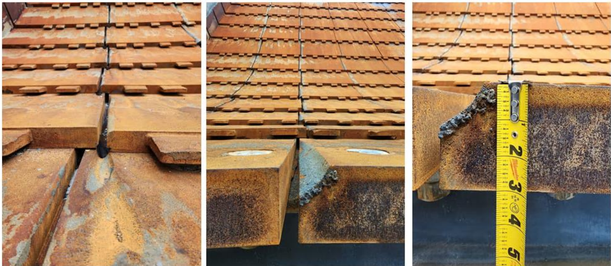
Figure 2. Artemis I Post Flight image of Ablation in Local Areas of Flame Deflector Plates
