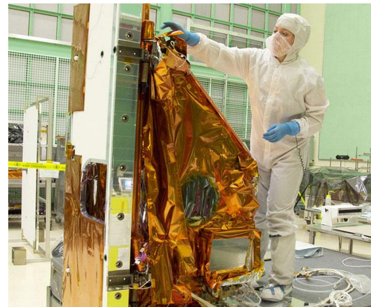
MLI blanket installation on TIRS instrument January 2012 (NASA)
