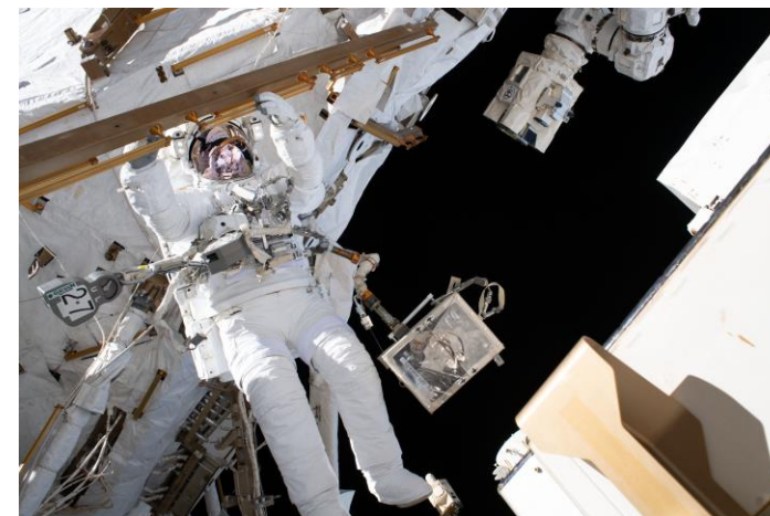
Gold anodized aluminum handrails as seen in spacewalk on January 2020 (NASA)
