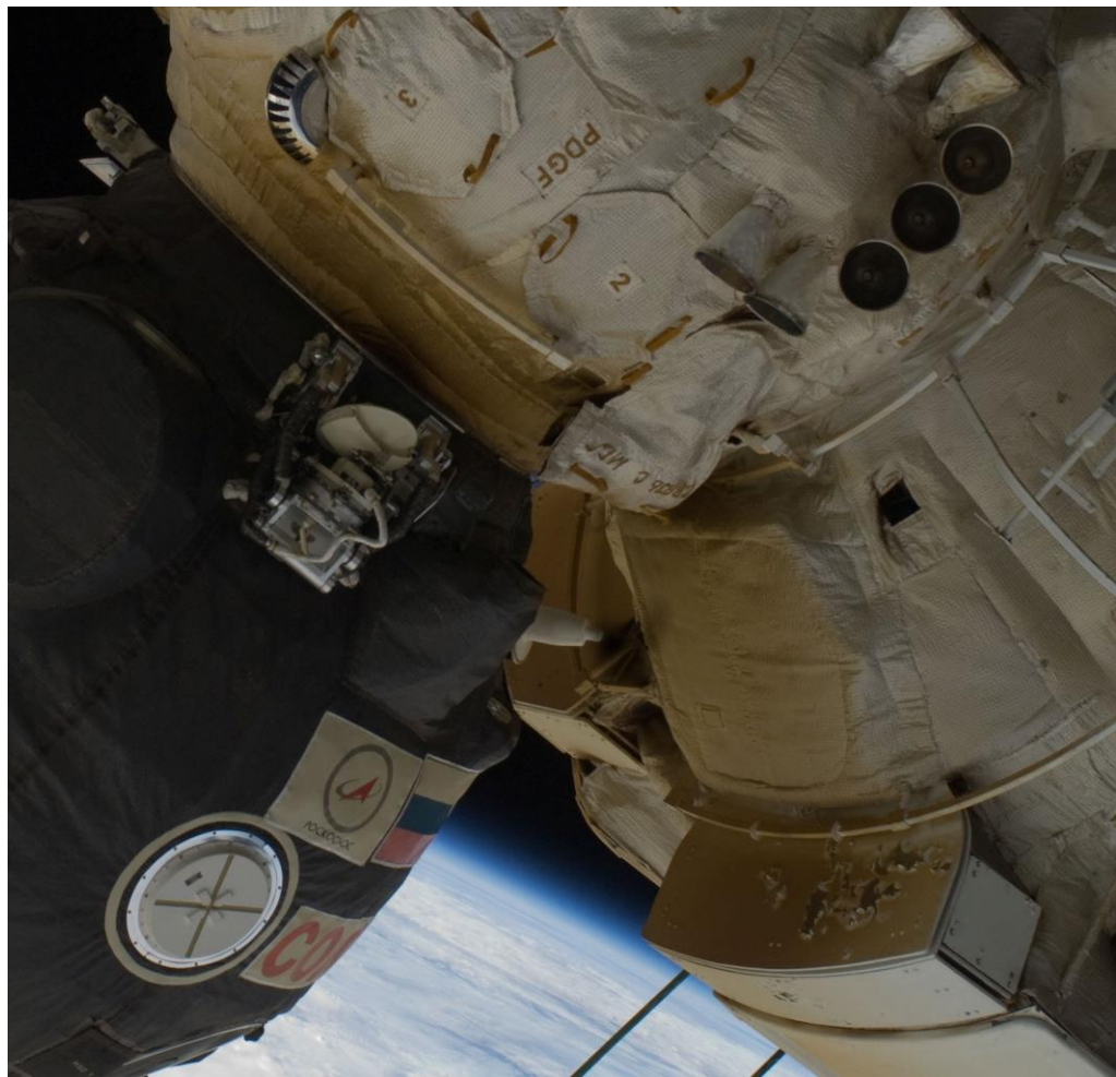
Contamination of thermal control surfaces seen on ISS Expedition 22 (NASA)
